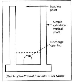
together with around 0.75 to 1.5 tons of fuelwood. The kiln is ignited and allowed to burn for approximately 48 hours and then cooled to recover about 0.75 to 1.5 tons of quicklime (CaO). Discharging is carried out from the bottom. Batch type kilns are normally used to burn coral and shell. Depending on capacity, the output of the kilns varies considerably.
